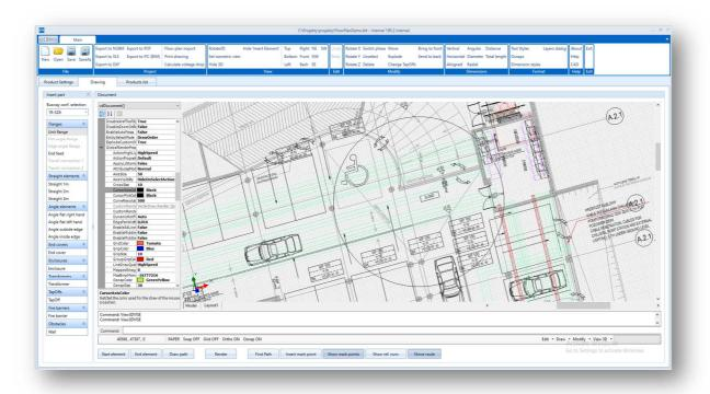
Most programs available on the market support the busbar layout design element by element, usually as add-ins to CAD applications. To meet requirements and focus on **Eaton Electric** products, we had to design a program that allows a **fast and effective** way to generate a busbar layout based on the **simple line drawing** (path), through which it is to be driven.
